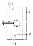
A signal proportional to the rotational speed of the motor can be generated with the mounted DST or DSA/20 speed sensor. The DST/DSA sensor registers the rotational speed and direction of rotation.
